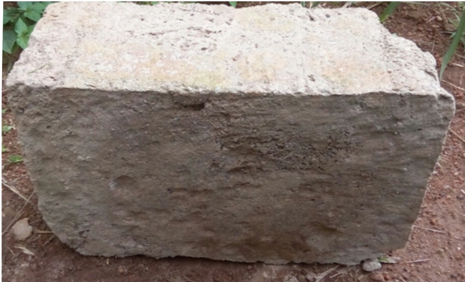
Plate 1: The Non-Hollow Block (Weight of 23kg with dimensions 0.23m x 0.15m).
