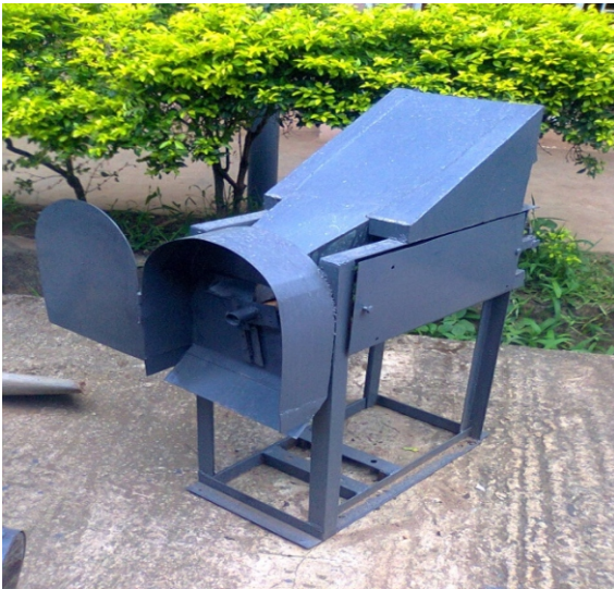
Plate 1: The fabricated leafy vegetable cutting machine
