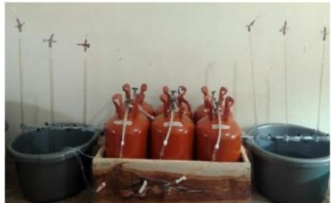
Plate II: Experimental set-up for studying the biogas yield from water hyacinth
