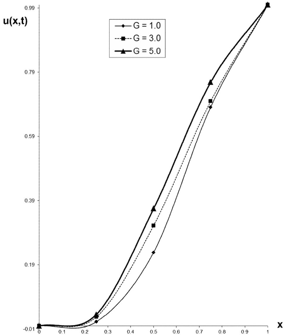
**Figure 3:**The graph of unsteady velocity distribution  $u(x,t)$  against  $x$  of a temperature dependent flow for equation 14 when  $P = 1.0, V_0 = -1.0, Ec = 1.0, a = 1.1, t = 0.2$  for various  $G$
