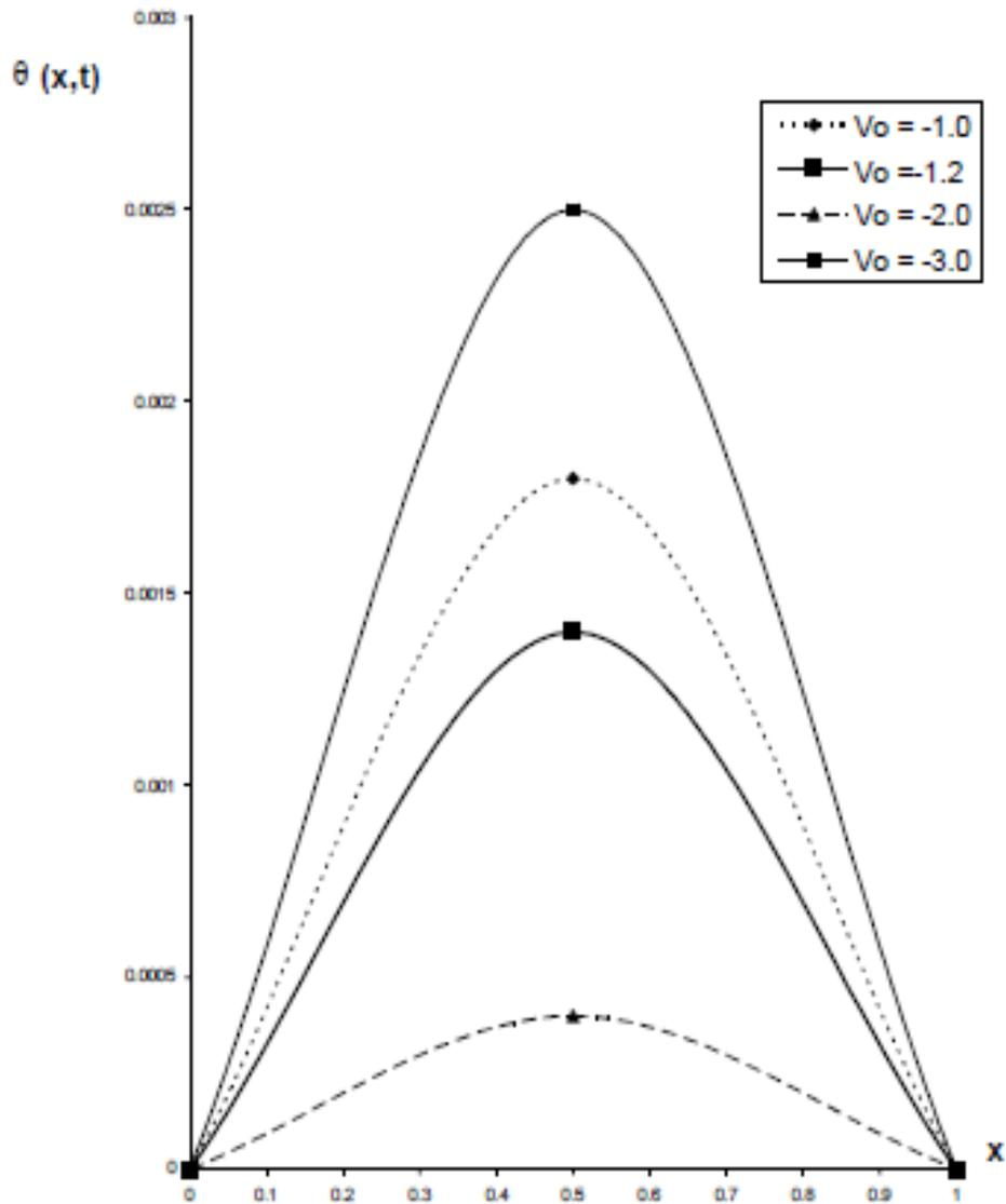
Figure 6: The graph of unsteady temperature distribution  $\theta(x,t)$  against  $x$  of a temperature dependent flow for equation 24 when  $P=1.0, Ec=1.0, a=1.0, t=0.2$  for various  $V_o$
