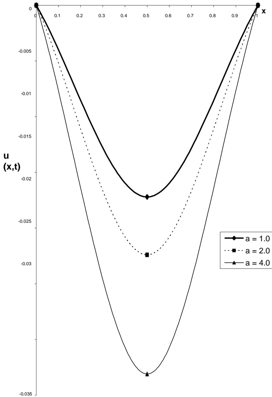
**Figure 4:**The graph of unsteady velocity distribution  $u(x,t)$  against  $x$  of a temperature dependent flow for equation 18 when  $P = 1.0, V_0 = -1.0, Ec = 1.0, t = 0.2$  for various  $a$
