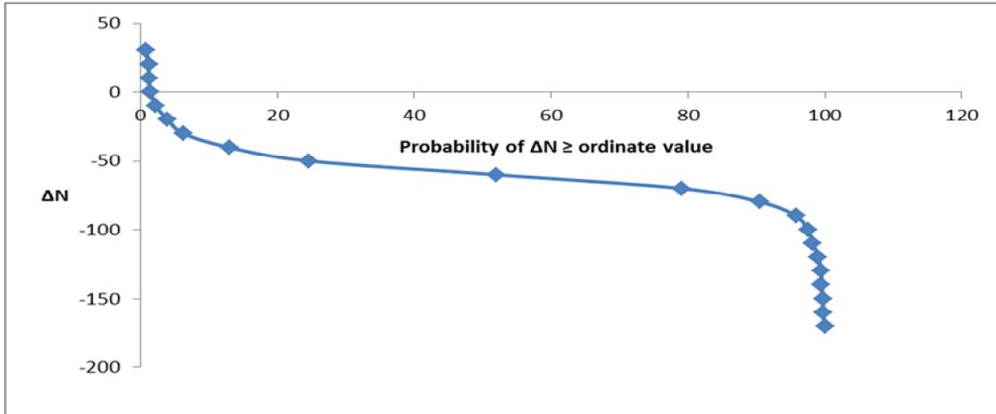
Figure 2: Cumulative Probability Distribution curve for the refractivity- gradients.
