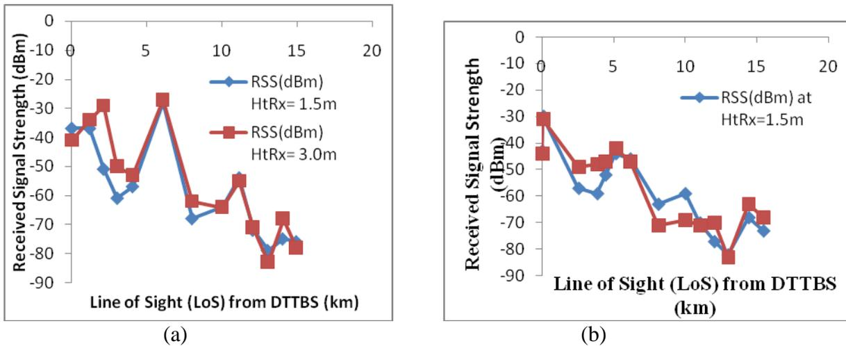
**Figure 5:** (a) Typical propagation curves for two receiver antenna heights during dry season in the year 2016 for Akure DTTBS. (b) Typical propagation curves for two receiver antenna heights during dry season in 2017 for Akure DTTBS
