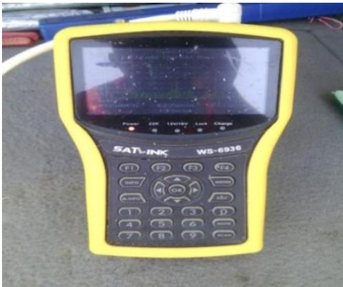
**Figure. 1: Digital field strength meter**
