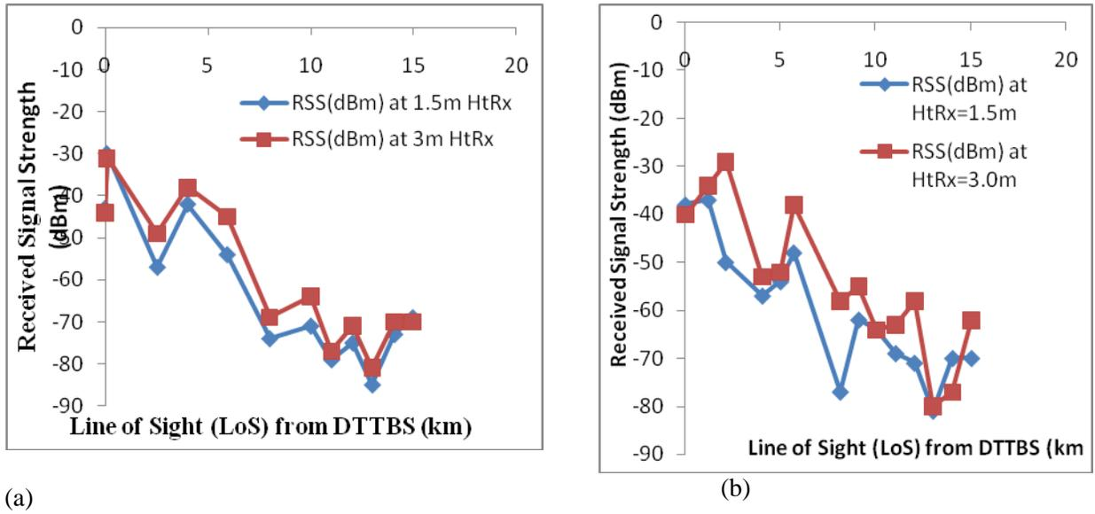
**Figure 6: (a) Typical propagation curves for two receiver antenna heights during wet season in the year 2016 for Akure DTTBS. (b) Typical propagation curves for two receiver antenna heights during wet season in the year 2017 for Akure DTTBS**
