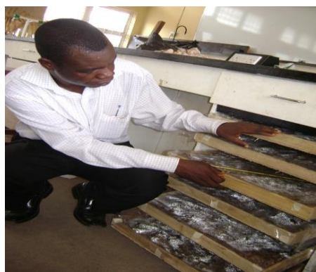
Plate 2: Fermentation chamber with the six-tier arrangement of the fermentation trays. The six trays were partly drawn out step-wisely to show the layered arrangement.
