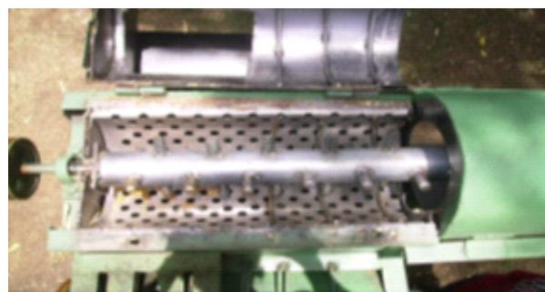
Plate 1: Cylinder concave configuration of the dual-crop sheller
