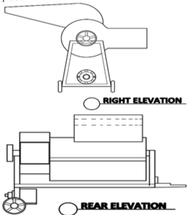
Fig. 4: Schematic representation of the right and rear elevation of the dual-crop sheller
