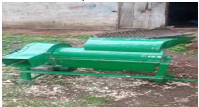
Plate 2: The fabricated dual-crop sheller
