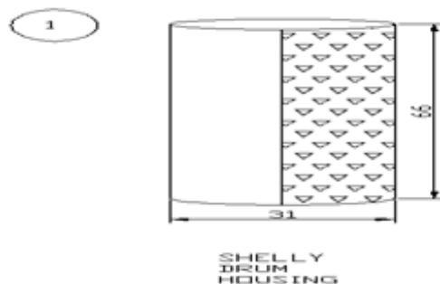
Figure 2: Removable perforated concave
