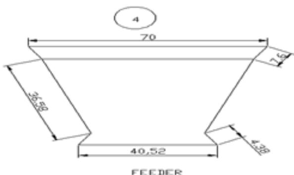
Figure.1: Schematic diagram of the hopper
