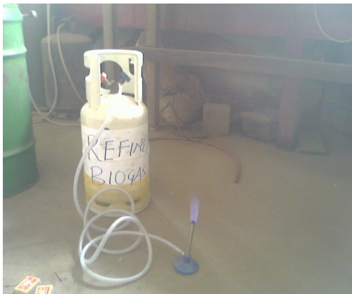
Plate 3: A picture showing the combustion of biogas from the cylinder
