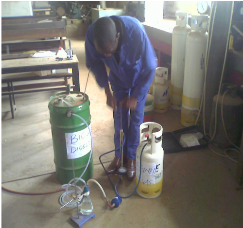
Plate 2: A picture showing the collection of biogas from the digester
