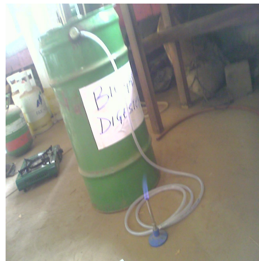
Plate 1: Test for burning of biogas from the digester
