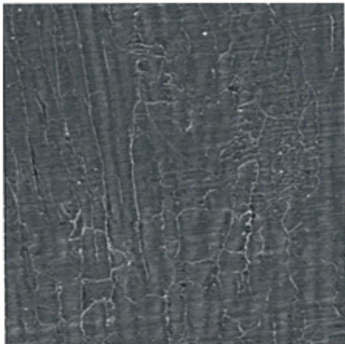
Fig. 3: Type A steel optical micrograph of WM welded with cellulosic coated electrode X100
